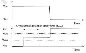
Figure 4. Overcurrent delay time
