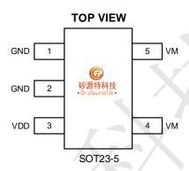
Figure 2. Pin Configuration
