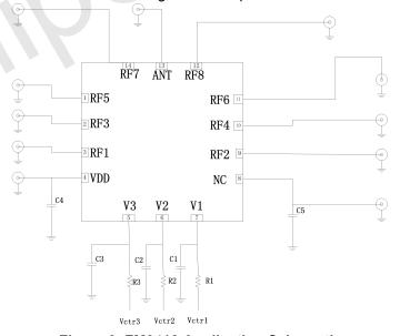
Figure 3. FM3418 Application Schematic
