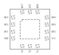
Figure 2. FM3418 Pinout - 14-Pin QFN (Top View)
