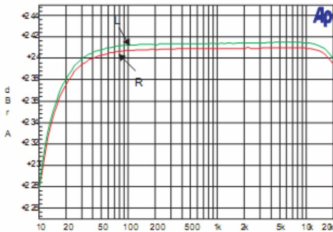
$V_{DD}=5V, R_L=8\Omega, \text{Gain} = 24\text{dB}, C_{in}=1\mu F$
