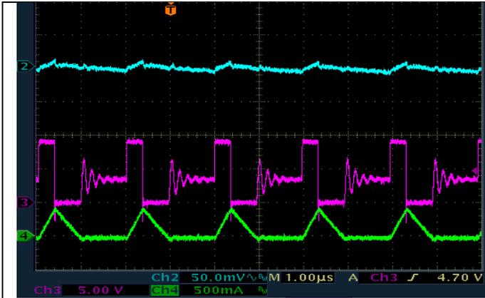
$V_{IN}=9V, V_{OUT}=3.3V, I_{OUT}=0.1A$
