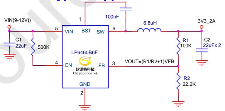
The C1 must be as close as possible to the chip, and the capacitor loop is the same.
