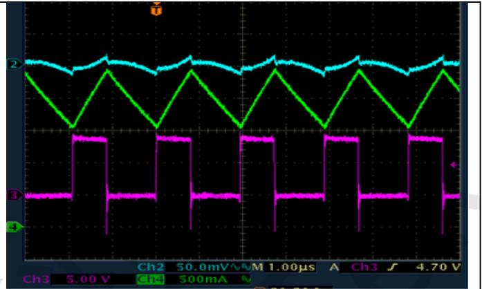
$V_{IN}=9V, V_{OUT}=3.3V, I_{OUT}=2.0A$
