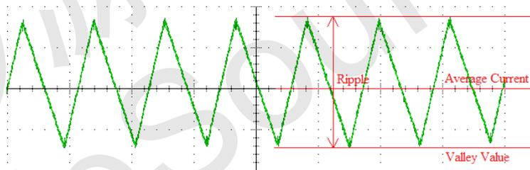
For example, as external components composed of 5V output, RY9120 uses 4.7uH inductance. Then the load capacity can be calculated when give 12V input supply.
