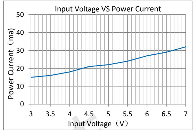
图6: Power Crrnt VS. Supply Voltage
